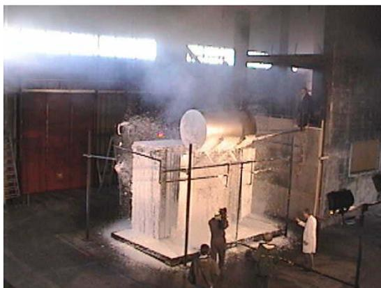
Figure 6 – Water Spray system vs CAF system for power transformer protection
