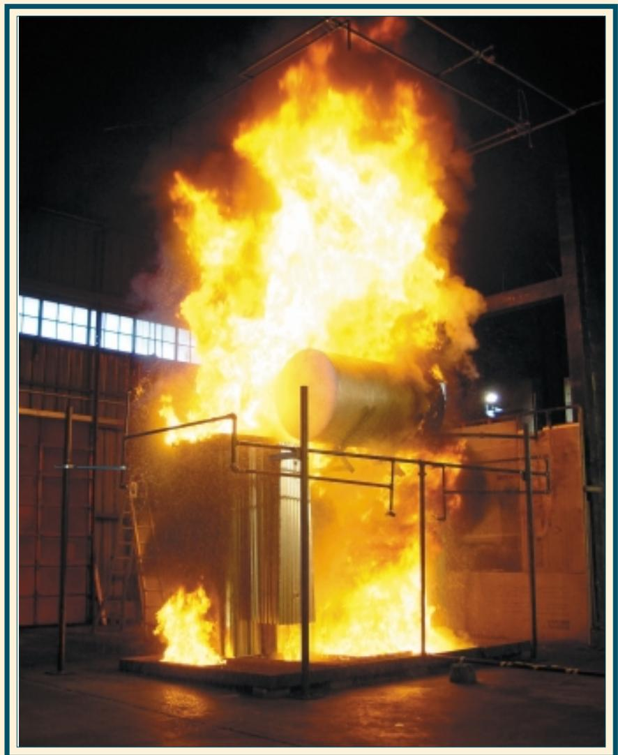
**Figure 4. Fully developed transformer fire**
