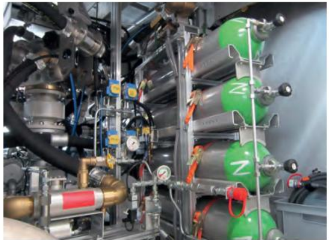
Pump / CAF compartment on Rosenbauer Panther ARFF vehicle at CPH
