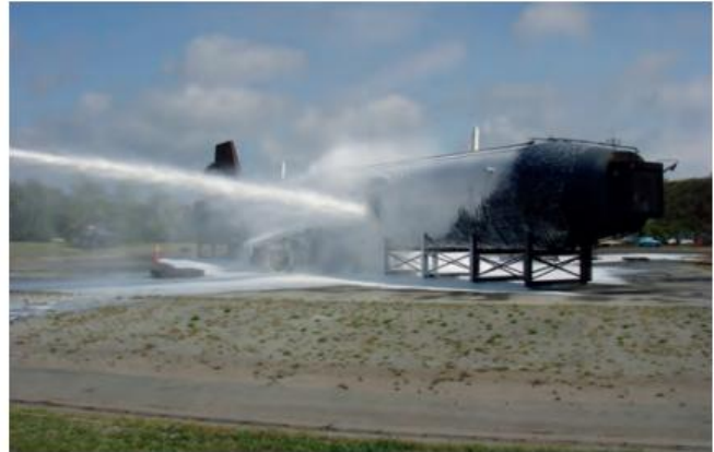
CAF discharge onto training prop at Copenhagen airport training facility
