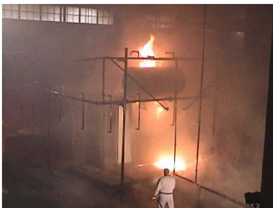
Figure 6 – Water Spray system vs CAF system for power transformer protection
