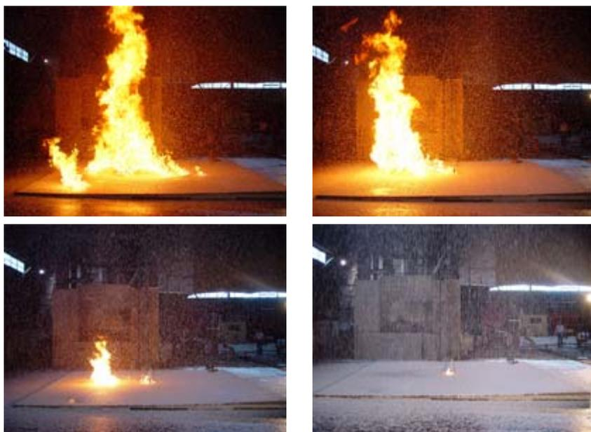
CAF extinguishes a free-flowing heptane spill fire in 38 seconds.
