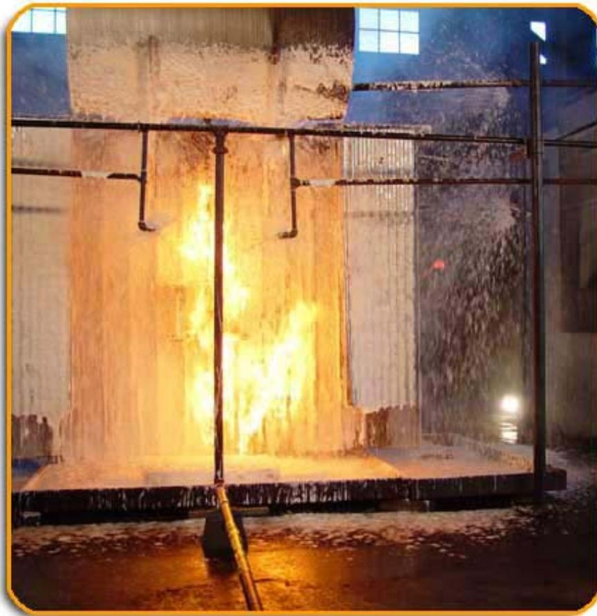
FireFlex's CAF-based system controlled a simulated power transformer fire in less than 45 seconds and fully extinguished the blaze in under 1.5 minutes. A traditional "deluge" type uses up to 10 times the water flow and is capable of extinguishing transformer fires in approximately 4 minutes. This tremendous water usage creates a large amount of hazardous waste caused by water mixing with contaminants from the transformer.
