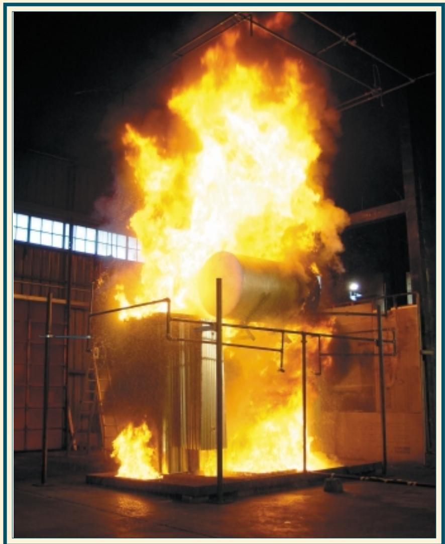
**Figure 4.** Fully developed transformer fire
