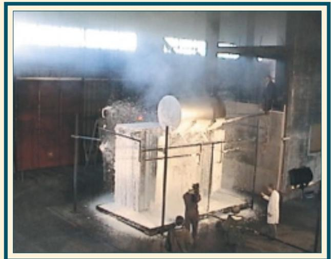
**Figure 5.** Water Spray system vs. CAF system for power transformer protection
